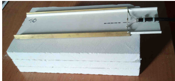
Fig. 4. Surface probe calibration for autoclaved calcium silicate
