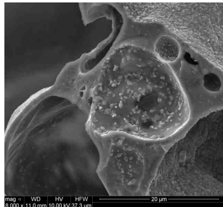
Fig. 4. Porous structure of lightweight aggregate fired at 1150°C, SEM above 8000x
