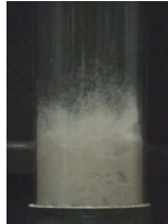
Fig. 3. The fluidised bed reactor just after the ignition of propane-air mixture (bed temperature 400°C)
