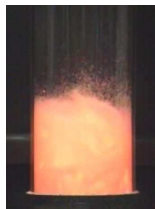
Fig. 4. The fluidised bed combustion of propane (bed temperature 900°C)
