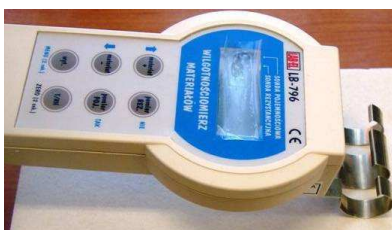
Fig. 1. Frequency Domain (capacitance) moisture meter (LAB-EL, Poland)
