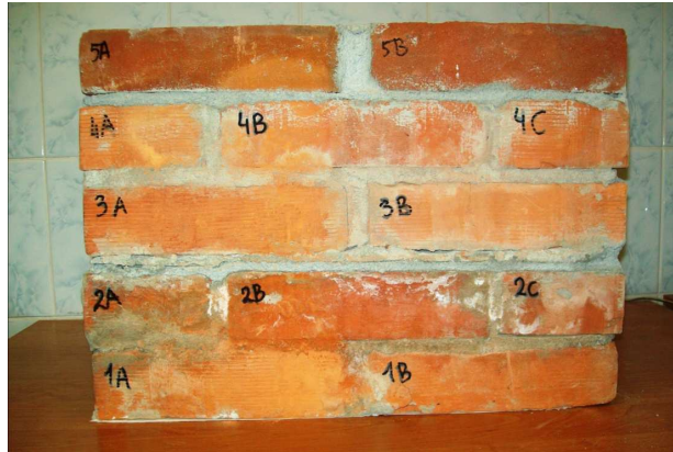
Fig. 3. Model wall made of red ceramic brick
