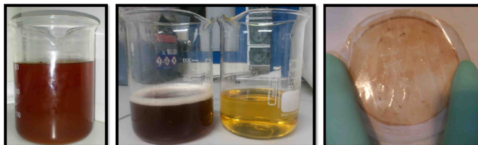
Fig. 7. Feed, permeate and concentrate and membrane after the process - UF-PES-5 membrane filtration
