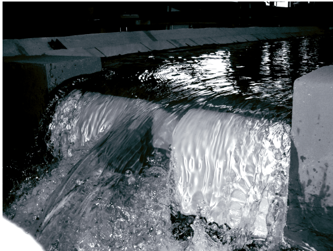
Fig. 4. Model of the Turawa measuring weir under laboratory investigation
