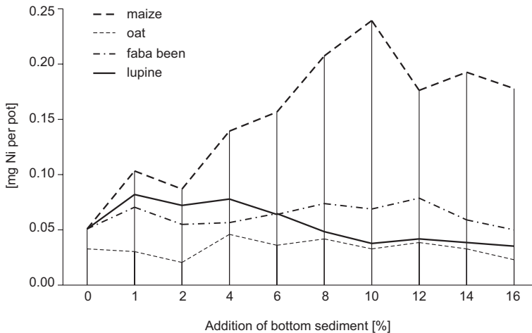
Fig. 3. Amount of Ni removed with yield of test plants depend on sediment addition to the substratum
