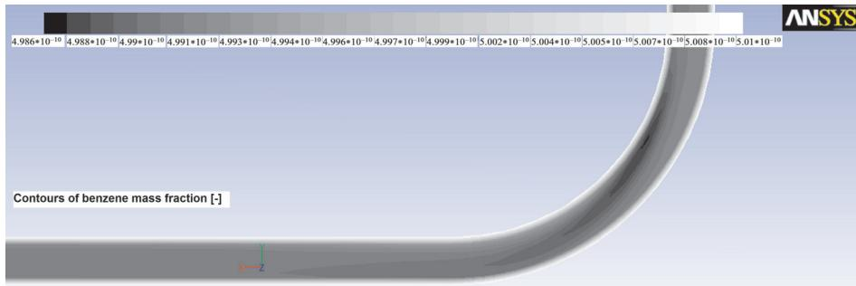
Fig. 3. The modeled benzene distribution inside water pipe: time duration 600s, mean flow velocity 1.5 m/s
