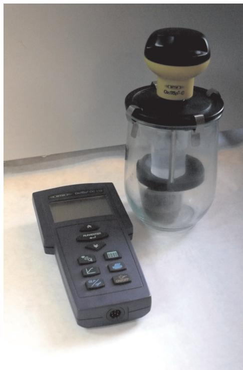
Fig. 2. A photo of equipment for measuring a demand for oxygen (photo: M. Kopeć)
