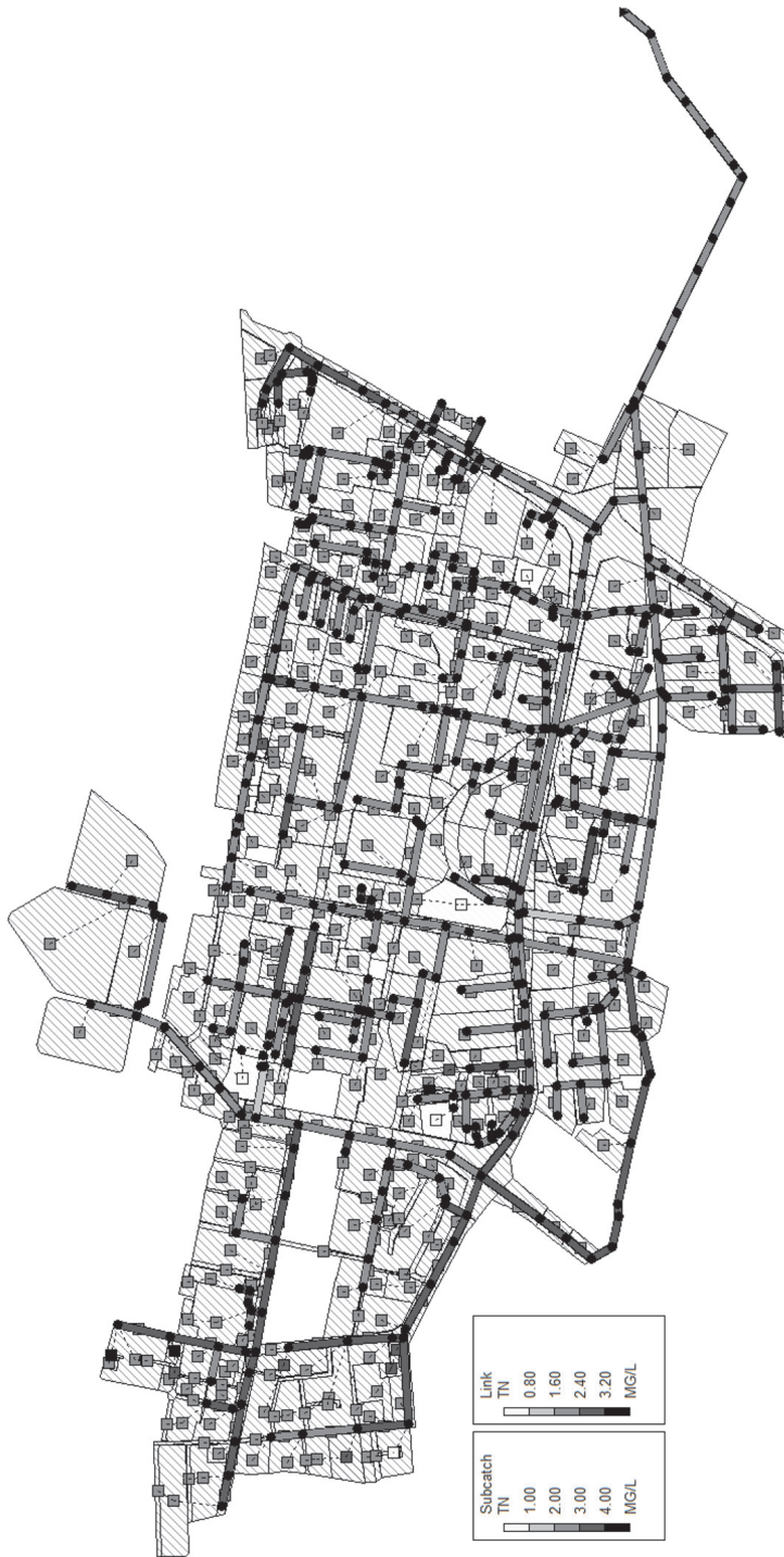
Fig. 8. TN concentration on subcatchments surface and in storm water pipelines
