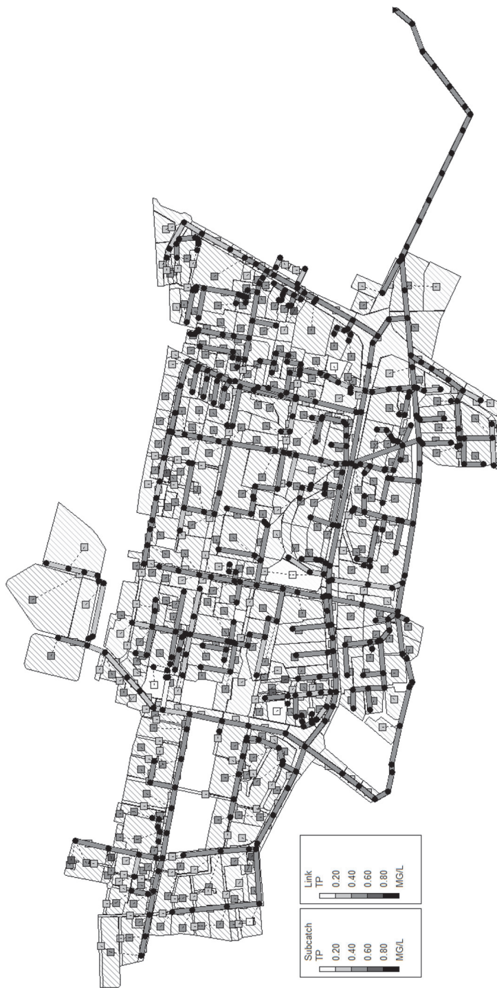
Fig. 7. TP concentration on subcatchments surface and in storm water pipelines
