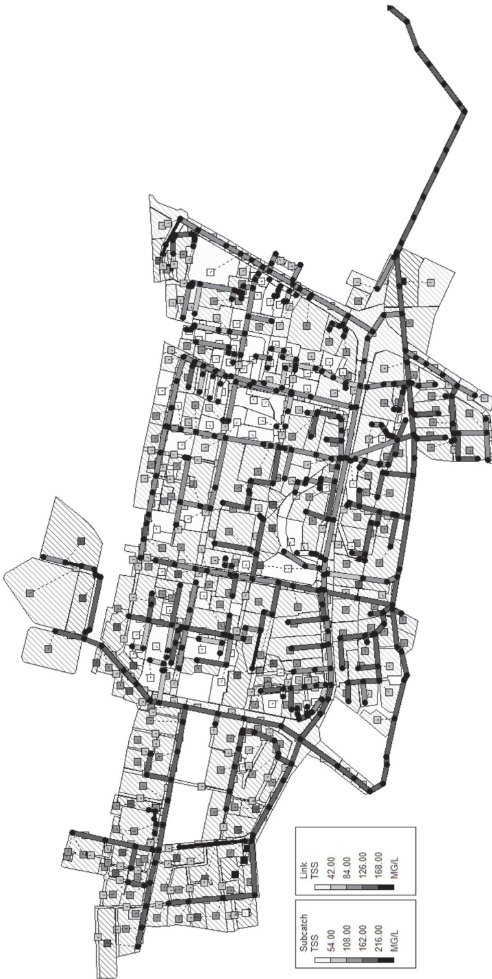
Fig. 6. TSS concentration on subcatchments surface and in storm water pipelines for Rain No III
