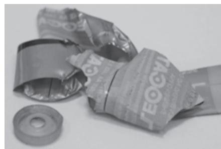
Fig. 4b. Plastic casing of Zn-C battery
