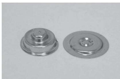
Fig. 2. Metallic collector +/- of Zn-C battery
