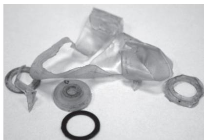
Fig. 7. Plastic spacer of Zn-C battery
