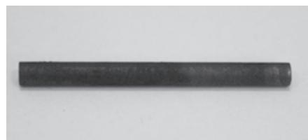
Fig. 3. Graphite collector of Zn-C battery
