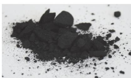
Fig. 5. Cathode mass of Zn-C battery
