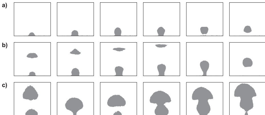
Fig. 5. Typical structures of bubbles formations a) spherical; b) pseudo-spherical; c) non-spherical
