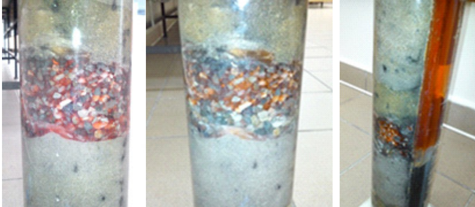
Fig. 4. LNAPL visible in the upper high permeable layer 1 day after its fourth addition (on the left) and 5 days after its fourth addition (in the middle and on the right [33])
