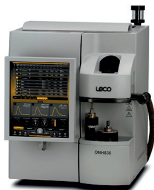
Fig. 2. LECO analyser of oxygen, nitrogen and hydrogen ONH836
