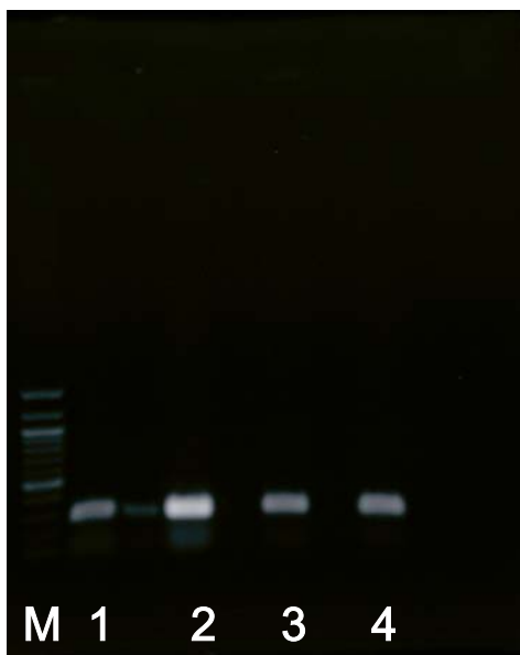
Fig. 1. Optimization of PCR for strain CCDM 128 by addition of 10 mM MgCl_2 to reaction mixture. M – molecular weight marker 100-bp DNA ladder, lane 1 – 0.4 mM, lane 2 – 0.6 mM, lane 3 – 0.8 mM, lane 4 – 1.0 mM MgCl_2
