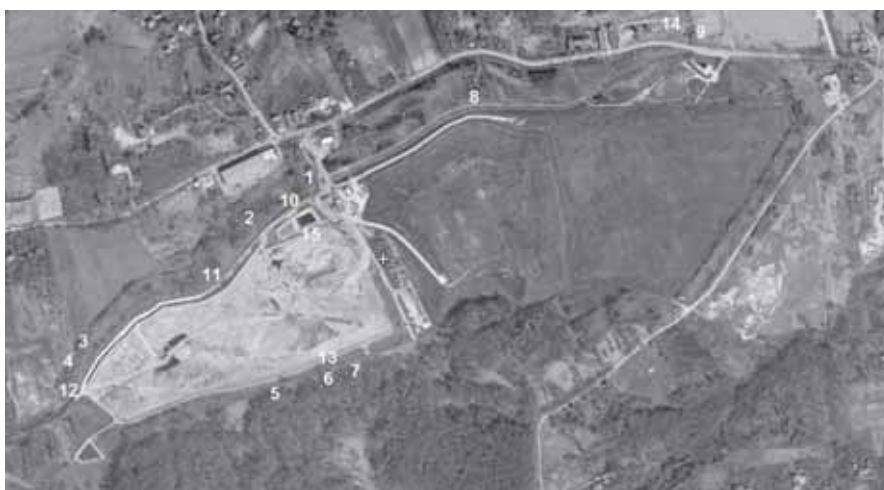
Fig. 1. Schematic layout of the research sites for water sampling at the municipal landfill Barycz in Krakow: 1–9 – groundwater research sites (piezometers), 10–14 – surface water research sites (Malinowka stream), 15 – leachate research site (working leachate reservoir) Source: Google Earth.
