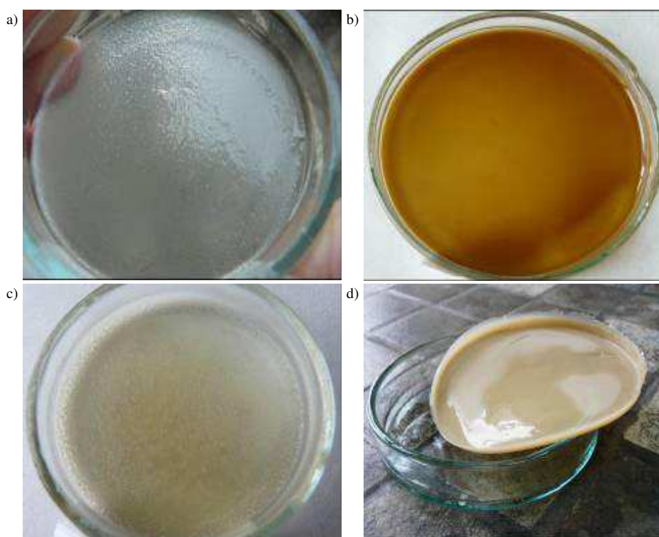
Fig. 1. Examples of alginate films: 1.5% alginic acid gel (a); non-defatted alginate film (b); defatted alginate film (c and d)
